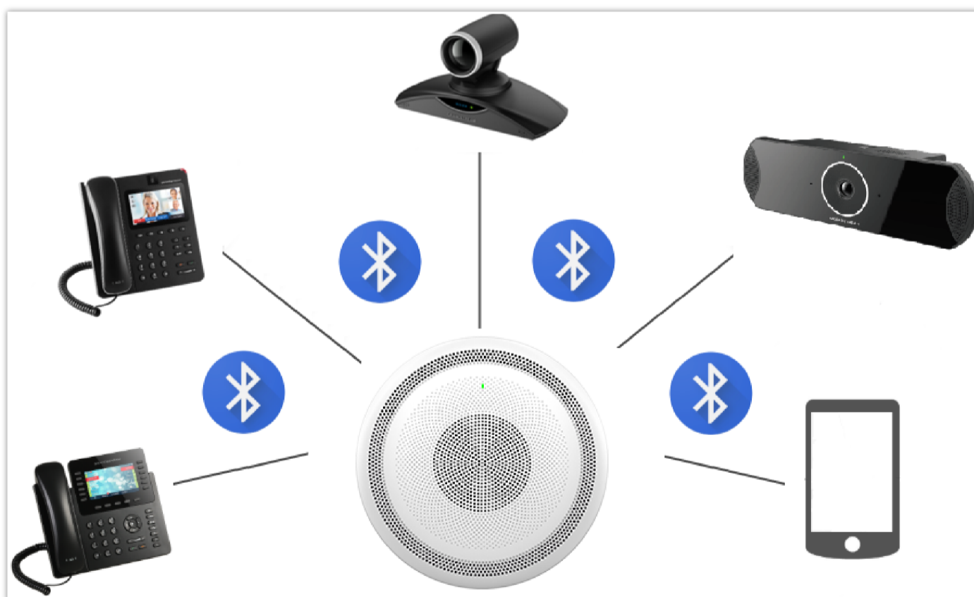
Connecting the GSC3516 as a Bluetooth Speaker
